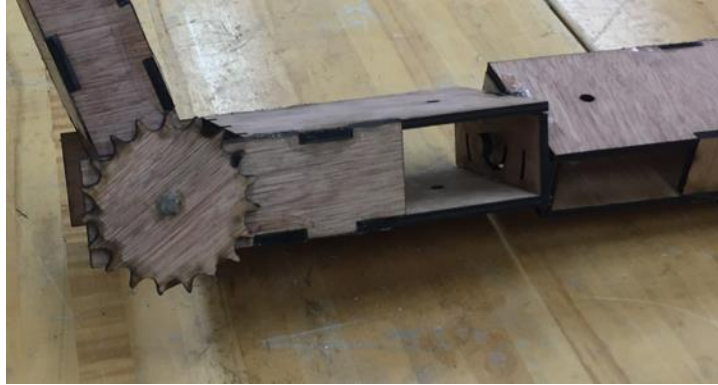
Figure 3. Second working prototype. It now includes a third DOF for rotation between modules.
